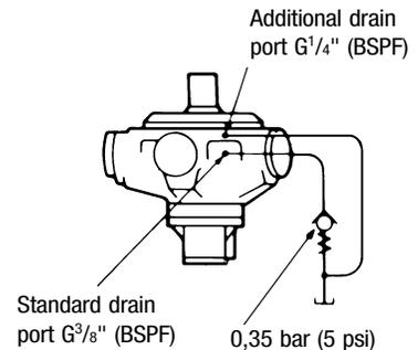
An additional drain port is provided when the “V” (shaft vertically upwards) designator is given after the shaft type letter in position **3** of the model code. This additional drain should be connected into the main motor casing drain line downstream of a 0,35 bar (5 psi) check valve to ensure lubrication of the upper bearing, see above diagram.
