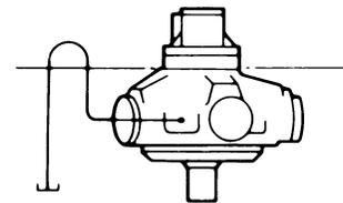
Use any drain position. The drain line should be run above the level of the uppermost bearing; if there is risk of siphoning then a siphon breaker should be fitted.
