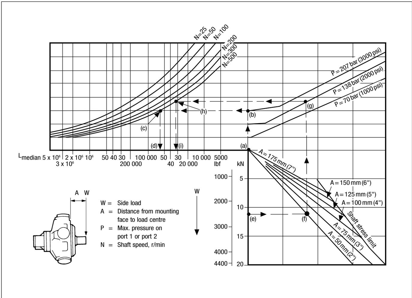
The nomograph allows the median bearing life to be determined for conditions of:
