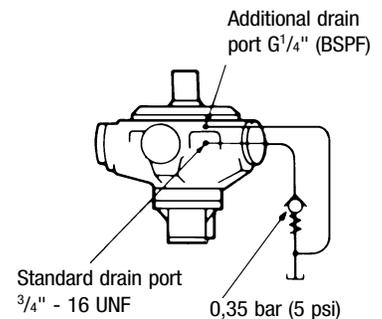
An additional G¼" (BSPF) drain port is provided when the “V” (shaft vertically upwards) designator is given after the shaft type letter in position **3** of the model code. This additional drain should be connected into the main motor casing drain line downstream of a 0,35 bar (5 psi) check valve to ensure lubrication of the upper bearing, see above diagram.
