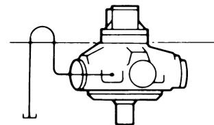
Use any drain position. The drain line should be run above the level of the uppermost bearing; if there is risk of siphoning then a syphon breaker should be fitted.
