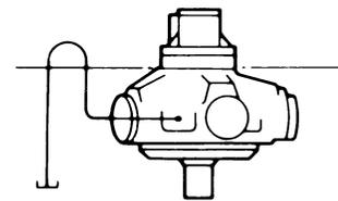
Use any drain position. The drain line should be run above the level of the uppermost bearing; if there is risk of siphoning then a syphon breaker should be fitted.
