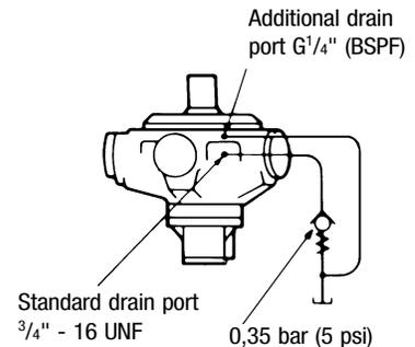
An additional G<sup>1</sup>/<sub>4</sub>" (BSPF) drain port is provided when the “V” (shaft vertically upwards) designator is given after the shaft type letter in position **3** of the model code. This additional drain should be connected into the main motor casing drain line downstream of a 0,35 bar (5 psi) check valve to ensure lubrication of the upper bearing, see above diagram.
