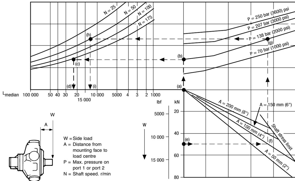
The nomographs on this and the following page allow the median bearing life to be determined for conditions of:
