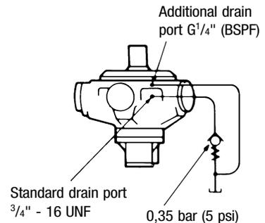
An additional G<sup>1</sup>/<sub>4</sub>" (BSPF) drain port is provided when the “V” (shaft vertically upwards) designator is given after the shaft type letter in position **3** of the model code. This additional drain should be connected into the main motor casing drain line downstream of a 0,35 bar (5 psi) check valve to ensure lubrication of the upper bearing, see above diagram.
