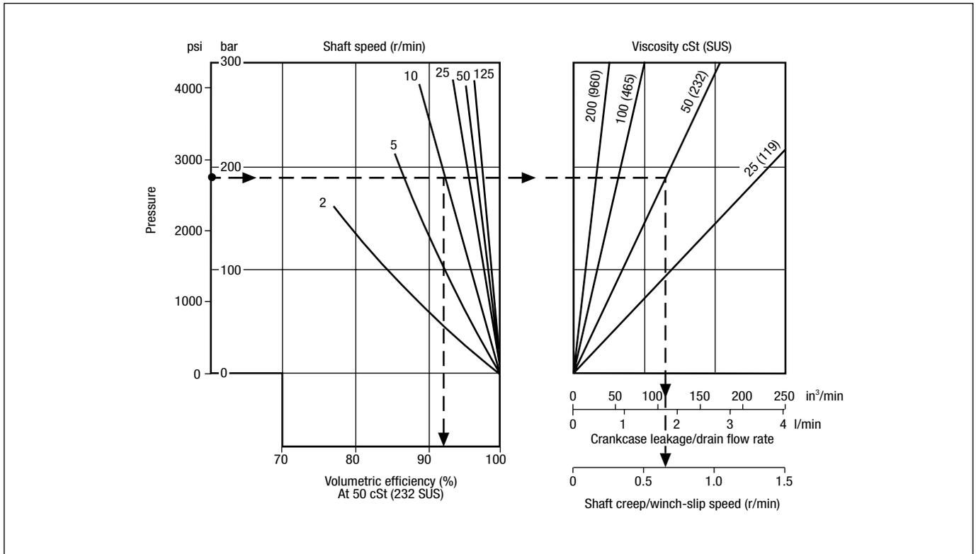
This nomograph enables the average volumetric efficiency, crankcase (drain) leakage and “winch slip”/shaft creep speed to be estimated.
