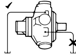
The crankcase drain must be taken from a position above the horizontal centre line of the motor.
